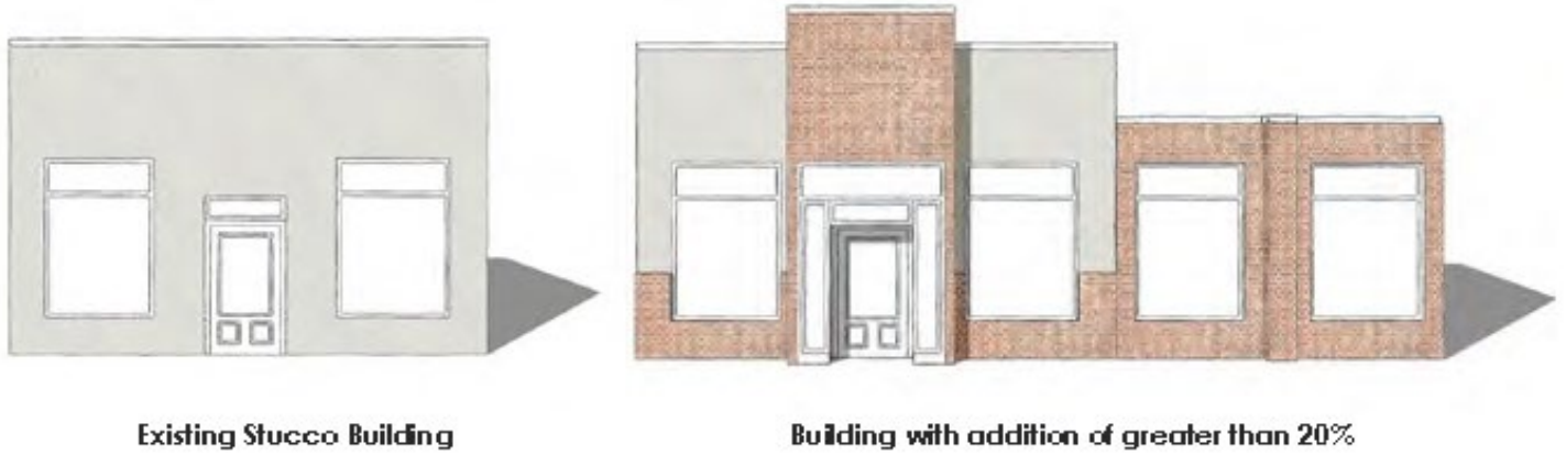
Figure 5.1 Example of Building Expansion Design Compliance
